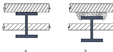
Figure 2: the steel structure is exposed to water from the outside (horizontal cross-section)
