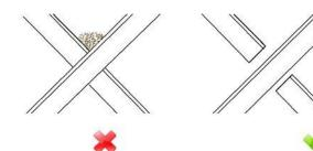
Figure 3c - Prevent water and dirt from remaining behind on joints by means of breaks
